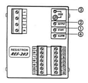
element and then subsequently reduced by the phase "chopping" action of the controller as soon as the preset temperature is reached. The high frequency of sampling together with virtually instant feedback gives the controller the high response control capability. The controlling action is indicated by LED (2)"OUTPUT", which changes its intensity with the change in voltage output. When more heat is needed, as in heating up or sealing, the LED is brighter.(also see Sect. 5.3)
