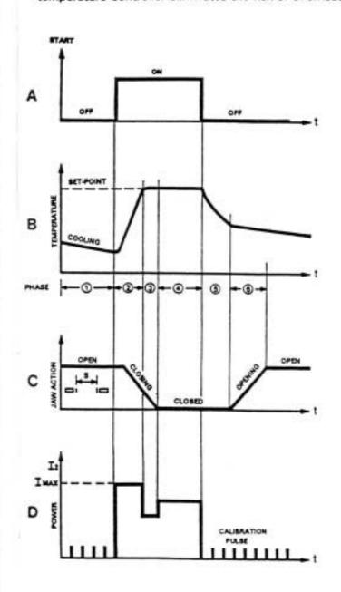
PHASE 1 - Power is "off". Jaws are "open" and the heatseal band is cooling from the previous cycle.
